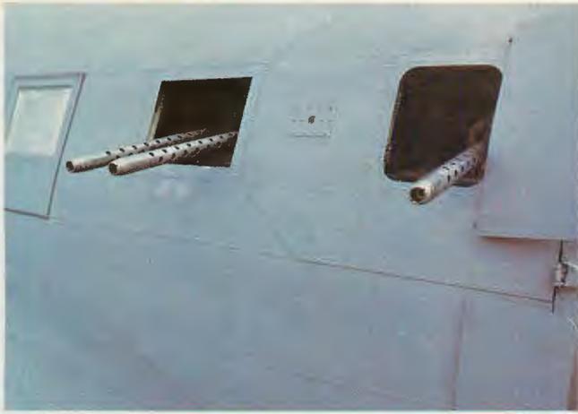
**ABOVE:** Three M3 .50-cal. Browning aircraft machine guns mounted in windows adjacent to left-side cargo door of AC-47.
